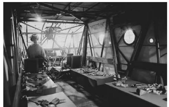
Fabric sides, no engine! Interior of WACO CG4-A glider configured for 13 troops. Typically towed by C-47, the 'Hadrian' could alternatively hold a jeep, a quarter ton truck, or a 75mm howitzer loaded through up-swung nose section. 15 companies produced total of 12,000. *-Brian Mahoney*
