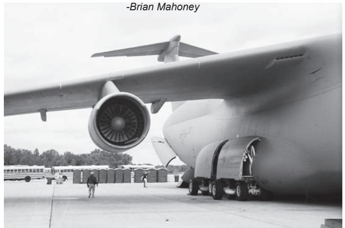
Crouching giant. Galaxy can lower to ground for the big heavy loads... note how high engine #3 is above grown man passing beneath. Main gear consists of 24 wheels in 6 trucks, nose has 4 wheels. Payload of 120 tons can go 5,500Km on one big drink of fuel.
